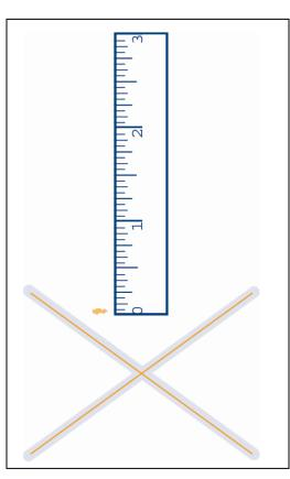
Paint chip is removed outside of the safety zone. This is a failure even if the chip is smaller than 1/16".
